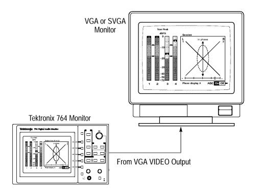
Figure 5: Using an external color monitor
